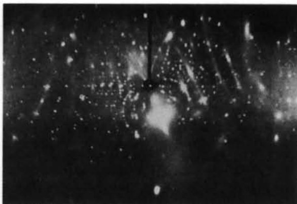
Fig. 1. Laue photograph, maleic acid, beam along the c axis, showing diffuse spots and streaks, especially very strong diffuse spot associated with 002. (Cu radiation, 30 kV., 15 mA., 2 hr.)
